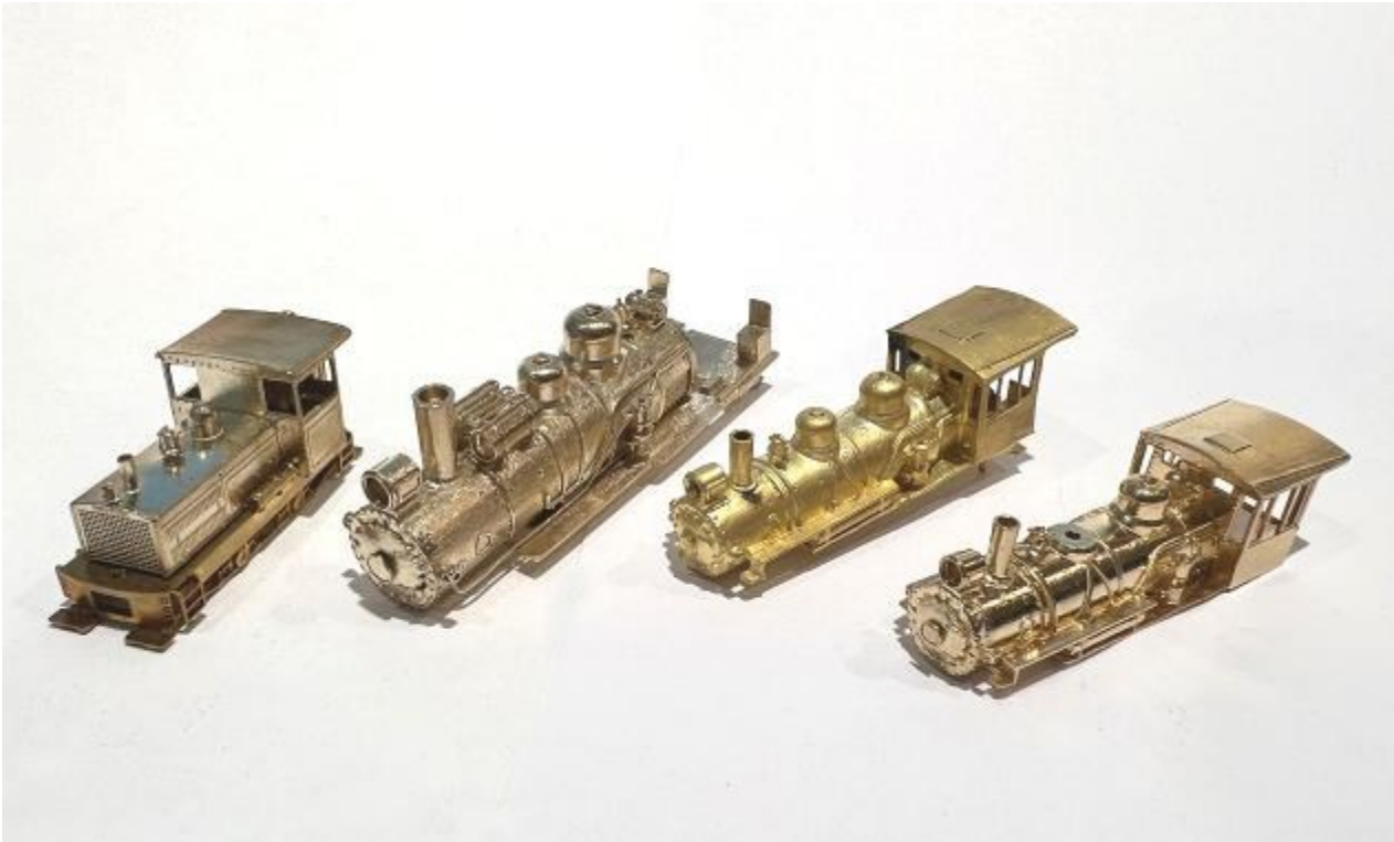
Brass lost-wax castings from 3D files, from left to right: Nn3 Plymouth HL 20 ton (Shapeways); TTn3 PCRy #110 boiler (Shapeways); Nn3 PCRy #107 (Trackside Details); Nn3 PCRy #107 (Sculpteo).
