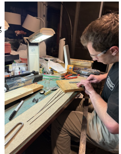
Dean Deis, fashioning the curved point / closure / wing rail for his first hand-laid switch. Linton von Beroldingen taught me how to hand-lay a switch in 1986; 40 years later I get to pass it on.
