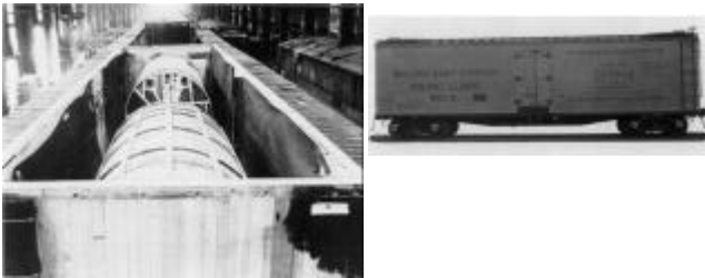
Fig. 8: Interior and exterior builder's photos of prototype 1X milk tank car
