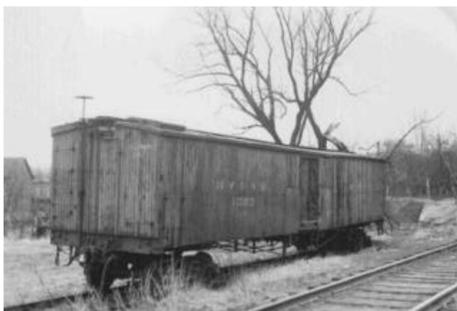
Fig. 5: Car No. 1023 photographed at Port Jervis on June 15, 1947 by Joseph A McLennan. Several details can be noted in the photo. The obvious sag was typical of many truss rod milk cars as the wooden under frame stressed from years of use. Note the herringbone pattern on the doors. COLLECTION OF JEFF OTTO
