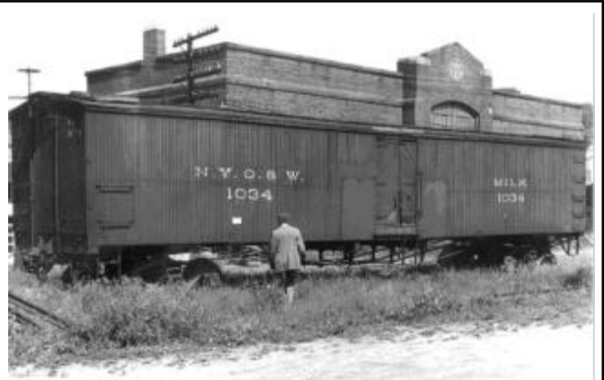
Fig. 6: Car No. 1034 photographed in Middletown by Hal Carstens in the late 1940s. Note the same herringbone door pattern as used on car no. 1023. The door sheathing was likely to have been bead board, a tongue and groove plank, with a decorative milled center bead. The rectangular feature to side the doors were steel plates, used to protect the exterior sheathing from damage during loading operations. The thrifty O&W would fabricate these plates from just about any available sheet steel and the size of the plates varied from car to car. By the time Hal photographed the well-preserved 1034, it was being used to store company records.
