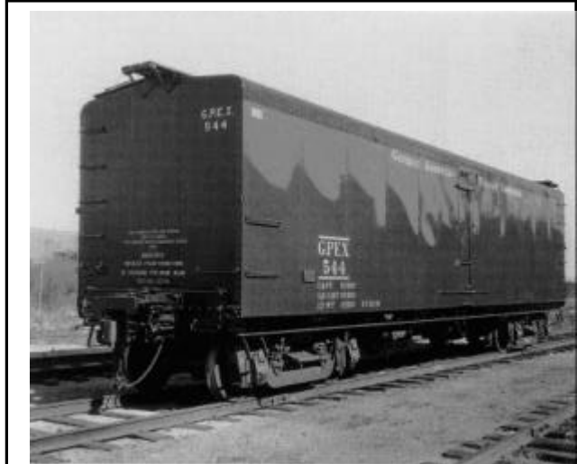
Fig. 12: The days of the double sheathed wooden milk cars were waning by the 1930s, as older GPEX cars began to be sheathed over in steel while newer cars were all steel construction.
