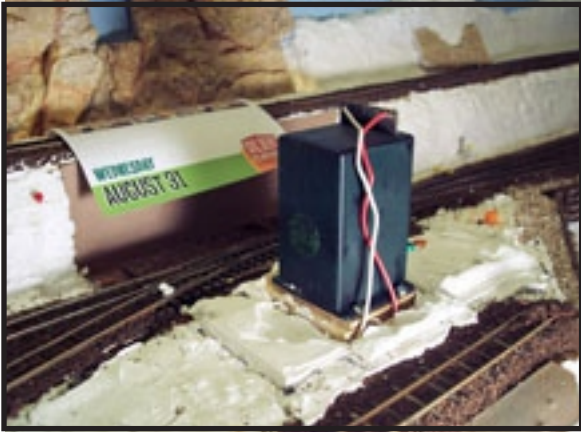
The problem – a surface mounted Tortoise switch machine on the very front edge of the layout's upper shelf.
