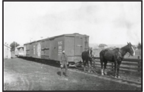
Motive power on the narrow-gauge Centerville Branch was provided by draft horses. Both of these cars appear to be combination box cars. These cars, which were built for fruit service, were equipped with two sets of doors, one solid wooden set for regular service and a second set made of iron bars to allow for ventilation. - Collection Bruce MacGregor
