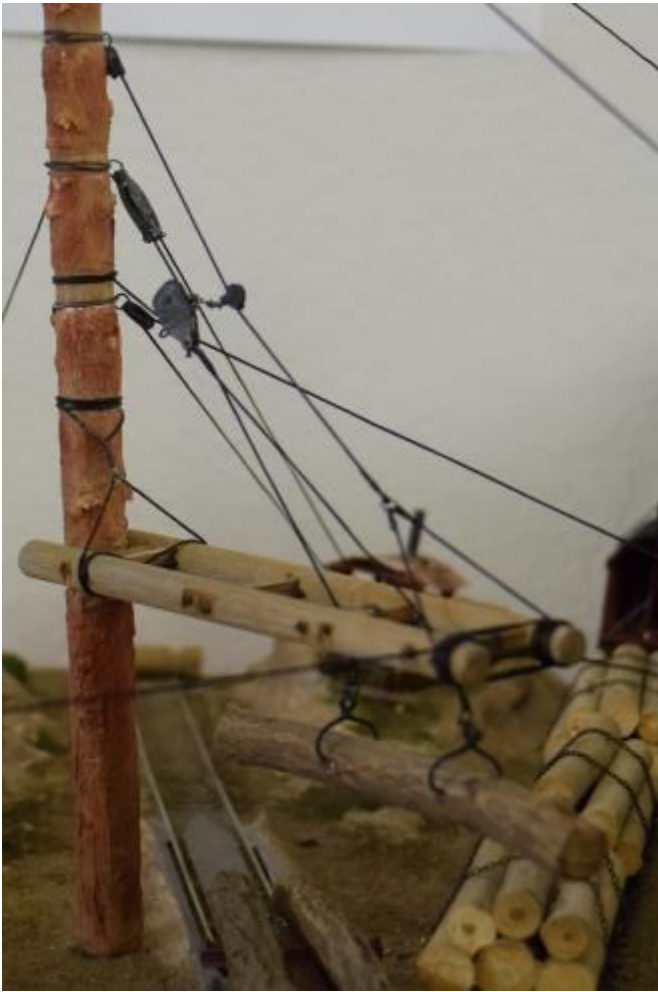
All Of The Blocks, Pulleys And Carriages On The Pole And Boom, Including The Log Tongs, Were Scratch Built From Styrene
