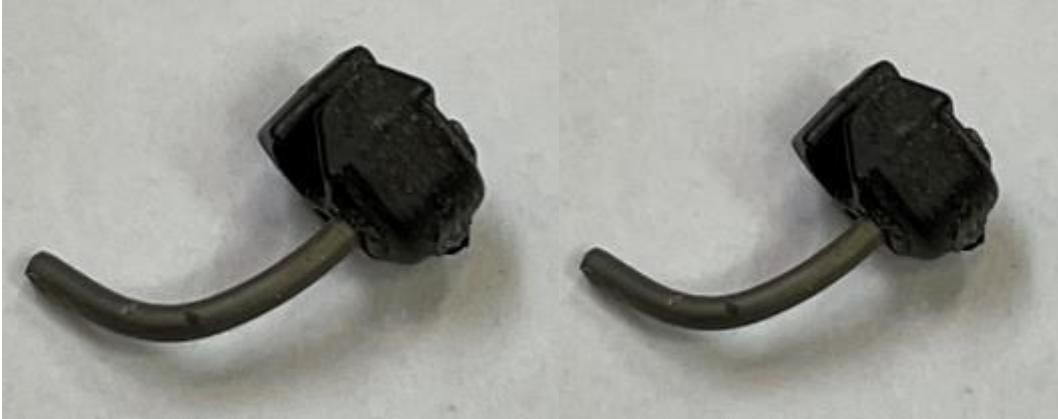
Couple shank(s) – we don't need situation cards; broken, bent... track/ train dynamics, buff and draft forces... they are real even on the model.
