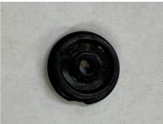
Wheel flanges are not indestructible. Plastic ones will chip, metal ones can crack or get welded to the rail.
