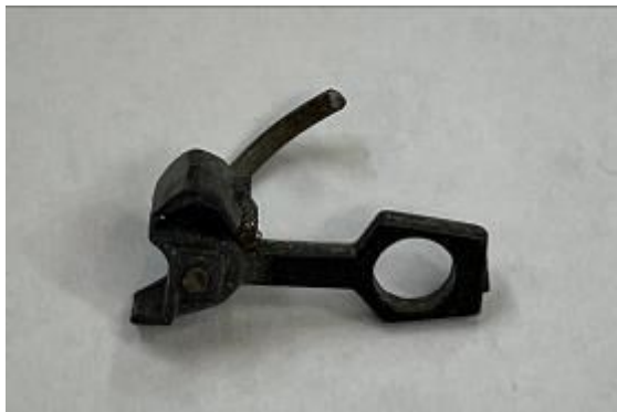
Broken knuckles – can't just carry a spare from the loco or caboose to fix the problem.
