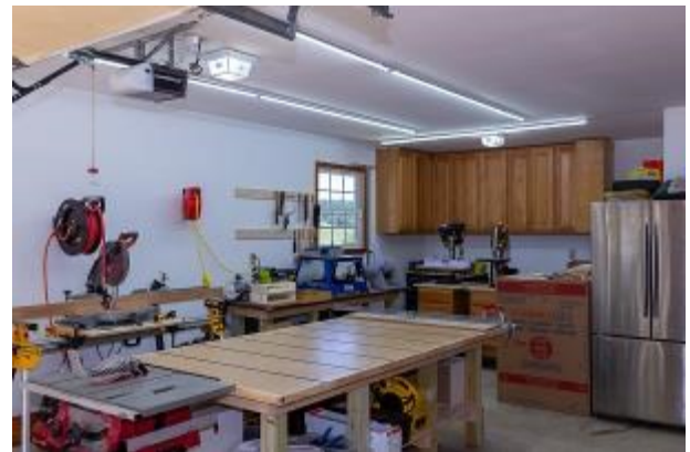
The garage workshop. This is where all the benchwork and supporting framework will be constructed. It includes a table saw, 12" miter saw, drill press, band saw, router table, bench grinder, vented spray paint booth, table-top belt sander and a 4'x8' assembly table.
