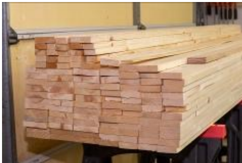
Additional lumber, 1x3, 1x4, and 2x4, are standing by ready to be cut to custom length L-Girders and cross members as construction gets started
