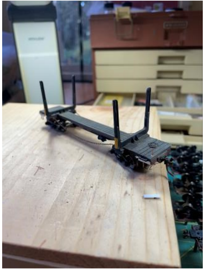
One of the skels with 'basic operating model' details – stirrup steps, brake wheel, cut levers, brake cylinder, air reservoir and triple valve are all in place. Brake rods and air lines will come later in the next level of upgrading the cars.
