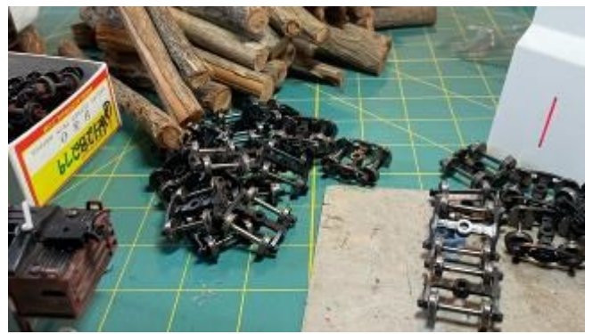
Center and right, trucks ready for installation. At left is one of the very old Mantua / Tyco / AHM gons with Kadee No 5 and coupler box installed. Just visible on the left is styrene glued into the body bolster so the new trucks can be mounted with 2-56 screws.
