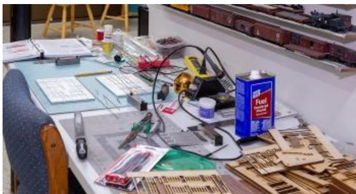
Hand-laid turnouts are built and adjusted at this workstation. Visible are a number of the Fast Tracks jigs, tools, and supplies.
