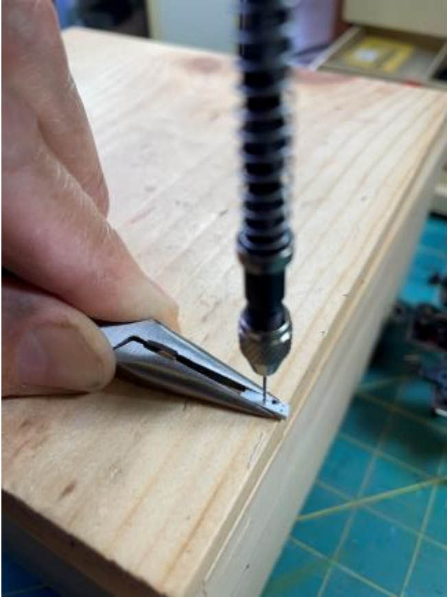
Drilling the 2x4 styrene for stirrup steps... I marked and drilled two holes in each 2x4 piece with a #74 bit to accept A Line #29000 Style A stirrup steps. Look closely at the photo. The first sill piece, which I marked with a black dot, is being used as a pattern for marking the rest.
