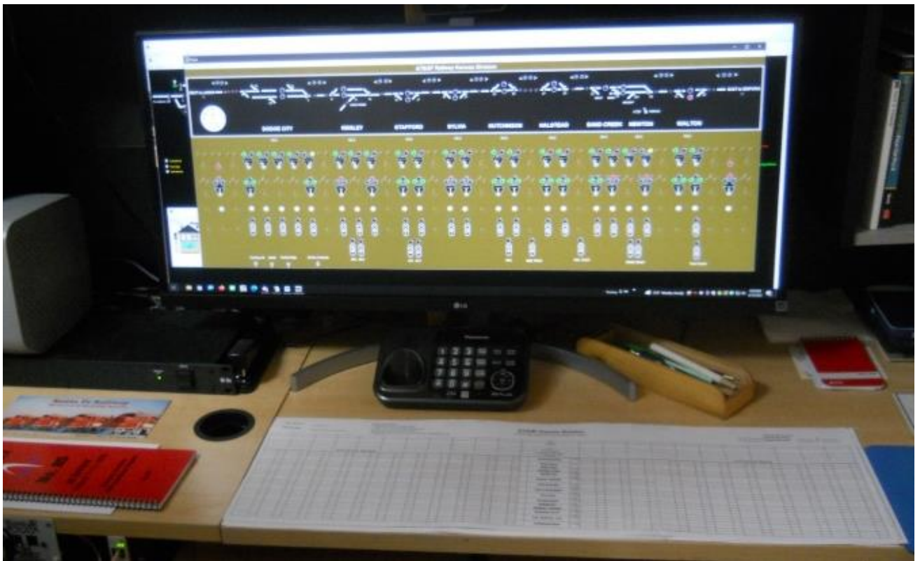
Dispatcher's station with CTC Panel and Train Sheet on Jay Janzen's Kansas Division
