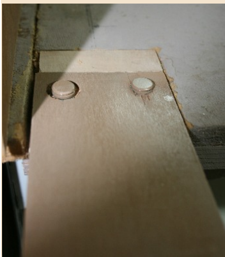
The lift-out gate, in place, rests on the benchwork, up against another piece of plywood, that is glued in place, so that the track can not move.
